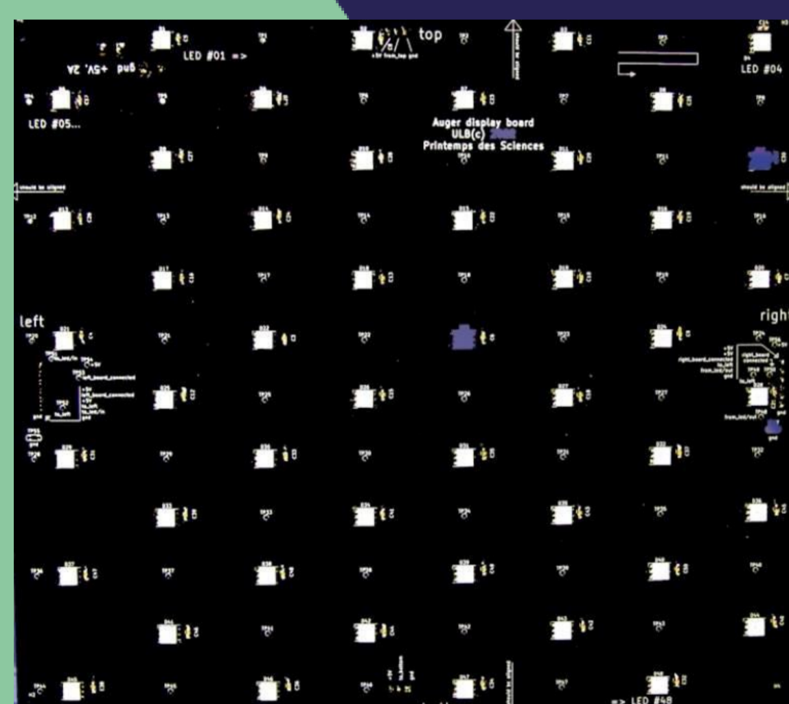
PCB contenant 48 LEDs (points blancs)
